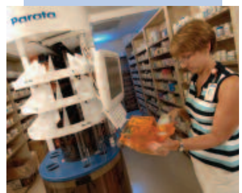
Parata RDS can fill a 30-count prescription in about 20 seconds.
