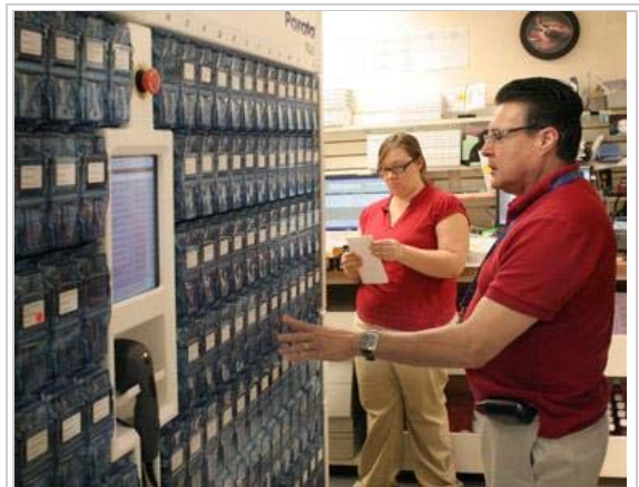
Steven King/Dispatch, Pharmacist Victor Provencia, right, demonstrates E.V.E., a robot that fills and dispenses prescriptions at the Sun Life Family Health Center in Casa Grande. By using the robot, errors in filling orders are reduced and efficiency is increased, allowing staff to focus their attention on the personal side of patient care.
